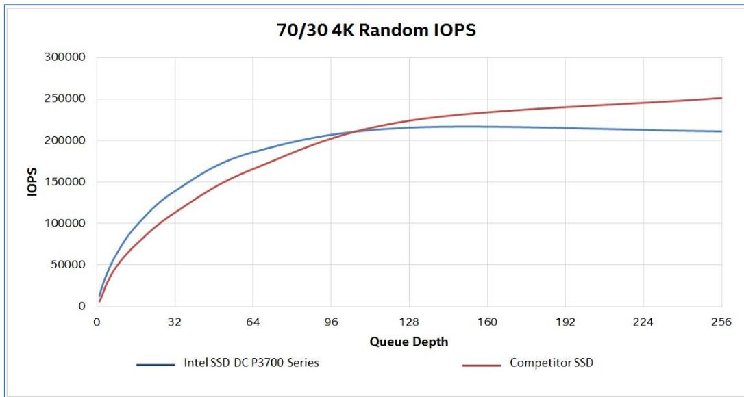
The above graph shows that as the queue depth increases, an increasing number of concurrent Flash components are utilized, thus increasing the performance. However, this increase is not linear with queue depth because random access will not distribute perfectly across the multiple dies in the SSD. As queue depth increases, there are more cases of commands landing on the same Flash component. As a result, the performance asymptotically approaches the saturation as the queue depth gets large.
