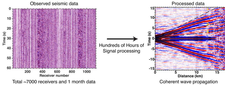
Figure 2. Effects of hundreds of hours of signal processing on observed seismic data.
