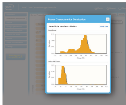
Figure 3. The detailed view of server power characteristics helps us increase rack density and properly design power capacity on the room, row, and rack levels.
