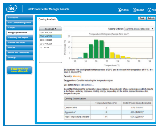
Figure 4. Intel® Data Center Manager's cooling analysis shows temperature measurement distribution in the data center.
