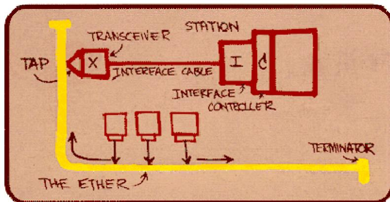
This diagram was hand drawn by Robert M. Metcalfe and photographed by Dave R. Boggs in 1976 to produce a 35mm slide used to present Ethernet to the National Computer Conference in June of that year. On the drawing are the original terms for describing Ethernet
