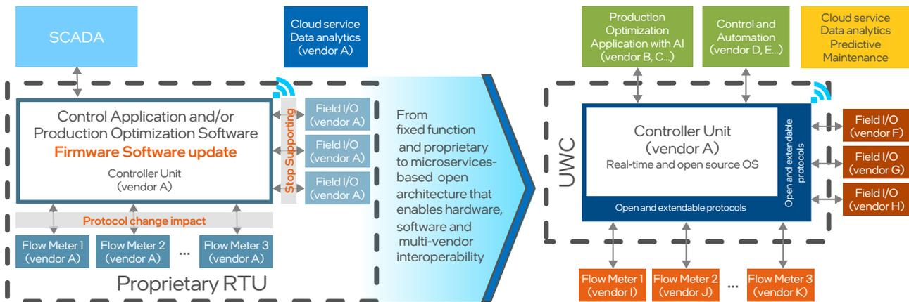
**Figure 1.** Industry transformation of traditional RTU-based proprietary technology to loosely coupled architecture with multi-vendor interoperability. The proprietary platform, from one “vendor A” shown on the left side, will be transformed into microservices-based control application over OTS hardware on the right side, delivering the protocol and multi-vendor interoperability, flexibility, scalability, manageability, etc. the O&G companies desire.
