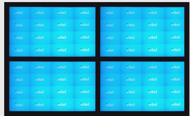
Figure 3: Using Intel® Core™ processors with integrated graphics, our example pipeline can support 64 streams being simultaneously decoded, resized, and composited into a video wall, playing at 22 FPS.
