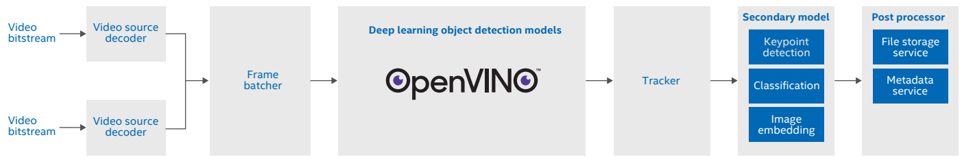
Figure 1. System architecture of ST Engineering's video analytics engine.
