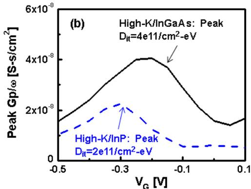
**Fig. 5(b):** Peak conductance measurements show low interface trap density,  $D_{it}$  (in low  $e11$  range) for both high-K/InP and high-K/InGaAs capacitors, although the latter shows 2X higher peak  $D_{it}$  value.
