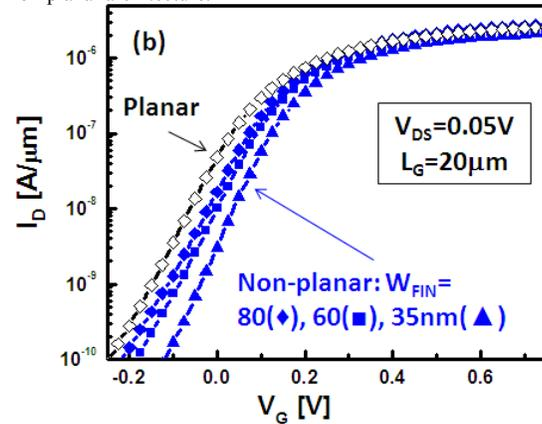
Fig. 9(b): Drain current ( $I_D$ ) versus  $V_G$  measurements on the same planar and non-planar QWFET structures as in Fig. 7(a). The data shows: (i) transistor threshold voltage ( $V_T$ ) increases, i.e. more enhancement mode, with reducing  $W_{FIN}$  due to stronger gate control, and (ii) subthreshold slope (SS) is low and similar for all the devices indicating good interface quality for all cases including the (110) InGaAs/high-K interface on both sides of the fin of the non-planar devices.
