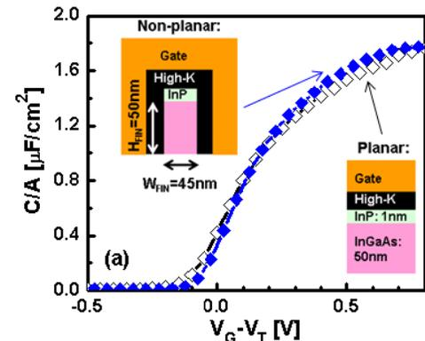
**Fig. 8(a):** C- $V_G$  measurements made on the planar and non-planar QWFET structures on the same wafer with same simplified  $n^{++}$  InGaAs S/D. The non-planar and planar structures have  $T_{OXE}$ =20.5Å and 21.5Å respectively. Similar to the planar structure, the non-planar structure shows healthy C-V characteristics with expected  $T_{OXE}$  indicating that the entire InGaAs fin is fully gated.
