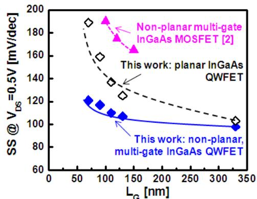
Fig. 12: SS versus  $L_G$  comparing the planar device (InGaAs QW thickness of 50nm) and non-planar, multi-gate QWFET device with  $W_{FIN}=60\text{nm}$  and  $H_{FIN}=50\text{nm}$ . The devices have  $T_{OXE}\sim 21\text{Å}$  and ultra-scaled  $L_{SIDE}$  of 5nm. Comparing to the planar device, the non-planar device shows significant improvement in SS due to improved electrostatics. Included is the most recent non-planar, multi-gate InGaAs MOSFET device from Ref. [2].
