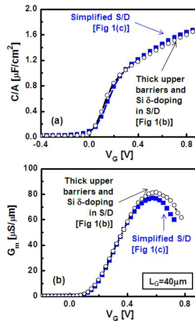
**Fig. 2:** Device structures in Fig. 1(b) and 1(c) show similar (a) capacitance (C) versus voltage (V<sub>G</sub>) and (b) transconductance (G<sub>m</sub>) versus V<sub>G</sub> characteristics, indicating that removal of thick upper barrier and Si δ-doping does not affect device performance adversely. This simplified S/D structure in Fig. 1(c) enables S/D contact area scaling with low resistance [5] and facilitates fabrication of the non-planar, multi-gate architecture in Fig. 1(d).
