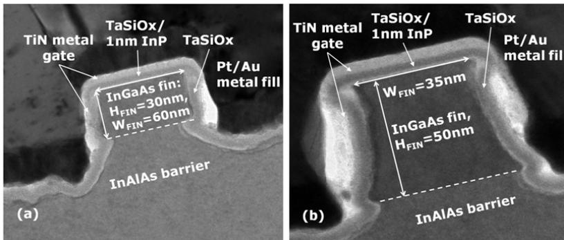
**Fig. 7(a)-(b):** TEM micrographs of two non-planar, multi-gate InGaAs QWFET device structures with different fin dimensions after high-K/metal gate formation. To ensure full electrical gating of the entire device, conformal ALD TaSiOx gate dielectric and PVD TiN gate metal are used.
