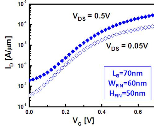
Fig. 10:  $I_D$ - $V_G$  of a non-planar, multi-gate InGaAs QWFET with  $L_G=70\text{nm}$ ,  $W_{FIN}=60\text{nm}$ ,  $H_{FIN}=50\text{nm}$ ,  $T_{OXE}=20.5\text{Å}$ , and  $L_{SIDE}=5\text{nm}$ .
