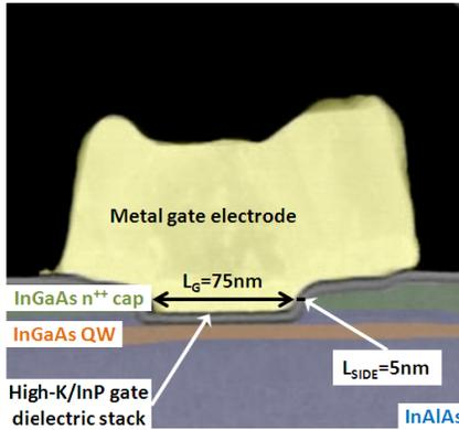
**Fig. 4:** Cross-section TEM micrograph of the non-planar QWFET showing the ultra-scaled gate-to-source/gate-to-drain separation ( $L_{SIDE}$ ) achieved via the TaSiOx gate dielectric layer.  $L_{SIDE}$  is determined by the physical thickness of the gate dielectric layer.
