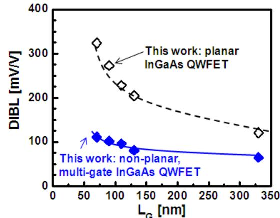
Fig. 11: Drain induced barrier lowering (DIBL) versus  $L_G$  comparing the planar device (InGaAs QW thickness of 50nm) and non-planar, multi-gate QWFET device with  $W_{FIN}=60\text{nm}$  and  $H_{FIN}=50\text{nm}$ . Comparing to the planar device, the non-planar device shows significant improvement in DIBL due to improved electrostatics.
