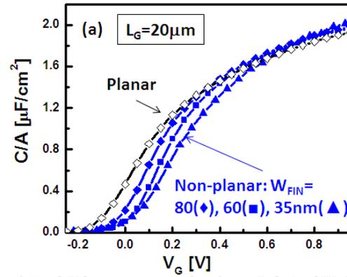
Fig. 9(a): C-VG measurements for planar (InGaAs QW thickness of 40nm) and non-planar QWFET structures with  $H_{FIN}=40\text{nm}$  and three different  $W_{FIN}=80\text{nm}$ ,  $60\text{nm}$  and  $35\text{nm}$  on the same wafer. All devices have long channel  $L_G=20\mu\text{m}$ . Similar to the planar structure, all three non-planar structure shows healthy C-V characteristics with expected  $T_{OXE}$  indicating that the entire InGaAs fin is fully gated.
