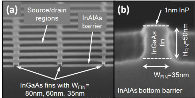
**Fig. 6:** (a) Tilted and (b) cross-sectional SEM micrographs of the InGaAs non-planar device structures after fin formation. In this work three different fin widths ( $W_{FIN}$ ) are used as shown in (a): 80nm, 60nm and 35nm. Fig. 6(b) shows an InGaAs fin structure with  $W_{FIN}$ =35nm and fin height ( $H_{FIN}$ )=50nm.
