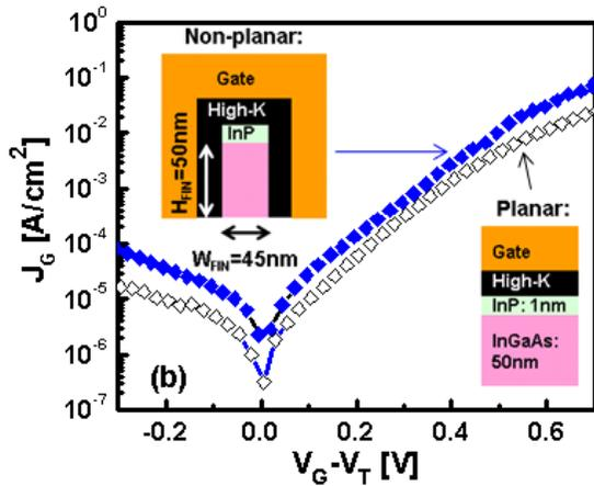
Fig. 8(b): Gate dielectric leakage ( $J_G$ ) versus  $V_G$  measurements made on the planar and non-planar QWFET structures as shown in Fig. 8(a). The non-planar QWFET structure shows similarly low  $J_G$  as the planar structure, indicating that there is no gate dielectric degradation in the non-planar architecture.
