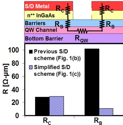
**Fig. 3:** Transfer length method (TLM) measurements show simplified S/D scheme in this work (Fig. 1(c)) achieves 90% reduction in barrier resistance ( $R_B$ ) over previous scheme (Fig. 1(b)), while  $n^{++}$  cap contact resistance ( $R_C$ ) remains identical as expected.
