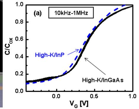
**Fig. 5(a):** C- $V_G$  measurements from 10kHz to 1MHz show minimal frequency dispersion for both high-K/InP and high-K/InGaAs capacitors, with good oxide quality on both substrates. The high-K gate dielectric is TaSiOx. The data suggests good oxide quality on both the top and the sides of the fin structure.
